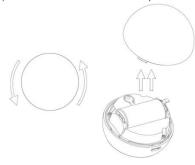
2) Remove the battery blocker.
